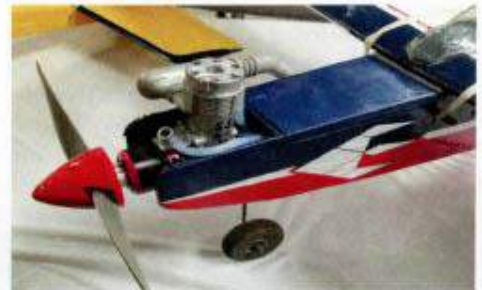
An electric Falcon with a dummy gas engine.
